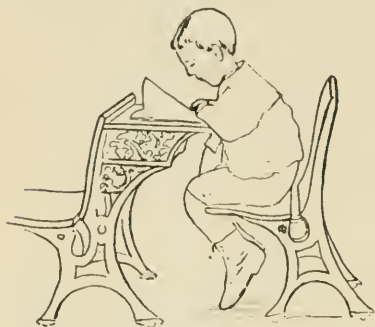
FIG. 39. — Illustrating a very common fault in school furniture, a too high seat. The child is unable to rest the limbs on the floor and leans over on the desk for support.
